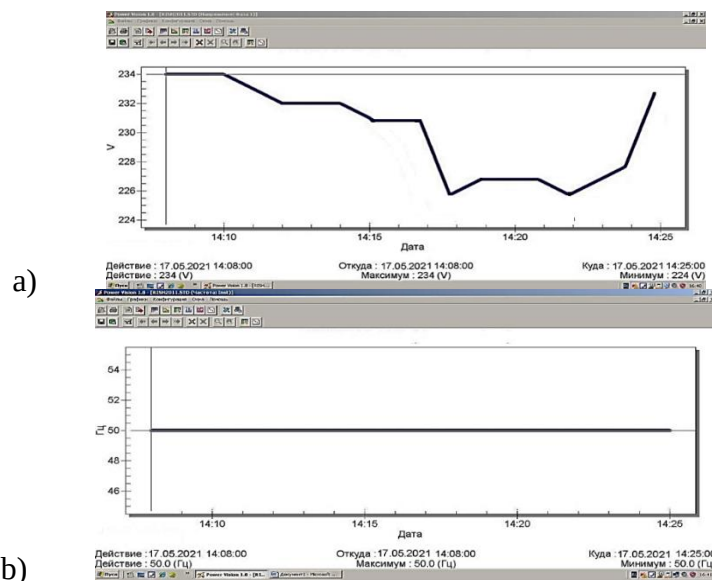
Figure 4. The analysis of the data obtained as a result of the test on voltage (a) deviation and frequency change (b) is presented
