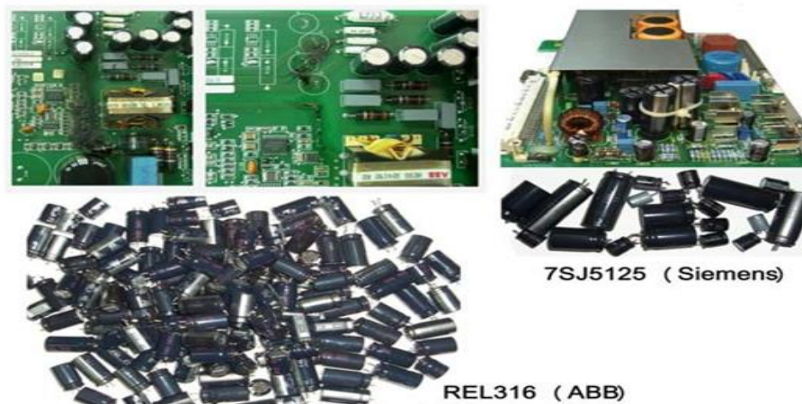
Fig. 1. Faulty DPR switched-mode power supplies of different types with damaged electrolytic capacitors. Left figure shows taints in printed circuit boards from electrolyte leakage.
