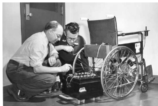
Pic. 8. Battery-charged wheelchair with electric motor created by Canadian inventor George Klein. 1950s
