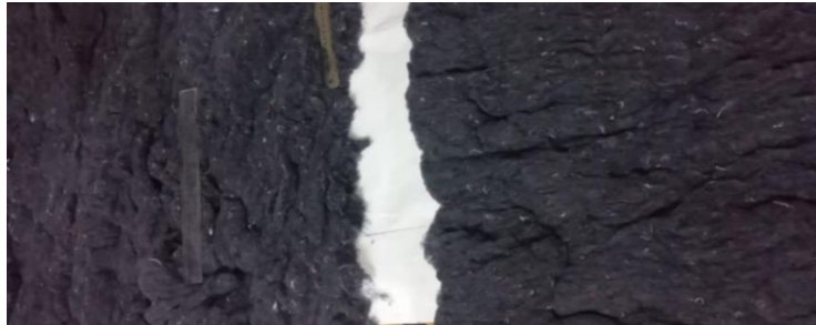
Figure 3. View of the fiber layer formed and separated in the punch drum.
