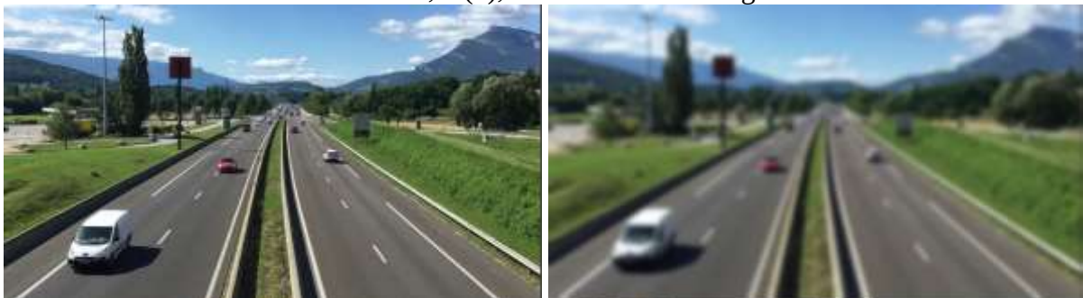
Figure 1. A simple image and the image after applying a Gaussian filter.
