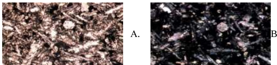
Fig. 2. Microstructure of basalt from the "Asmansay" deposit: left polarized, right transmitted light (magnification 150x).
