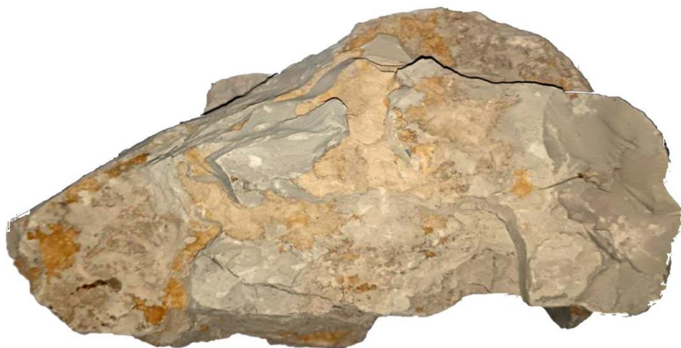
Figure 2. Geological sample of Ushsay bentonite clay
