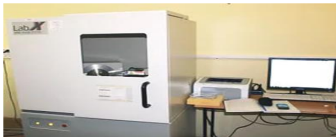
Figure 2. XRD-6100 X-ray diffractometer.
