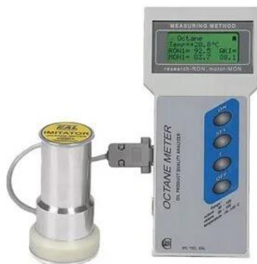
Figure 1. Overview of the Shatox SX-300 oil product quality determination device
